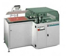
• The RIVOLINO is a multiple drilling and riveting system for the semi automatic riveting of the inner layers and prepregs to a multilayer.
